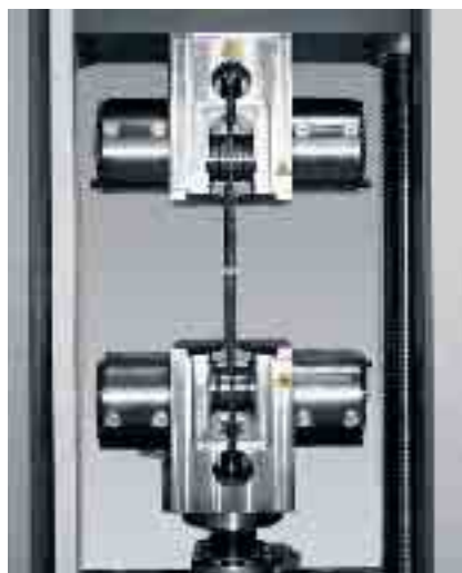
Hydraulic grips with dual clamping system (for strands e.c.)
