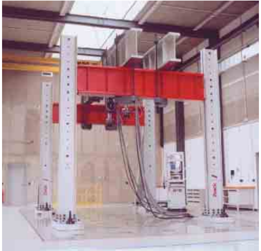
Component test system 1000 kN for the testing of supporting frameworks, large tubes etc. with a four-column load frame on an extremely rigid foundation plate made of reinforced concrete.
