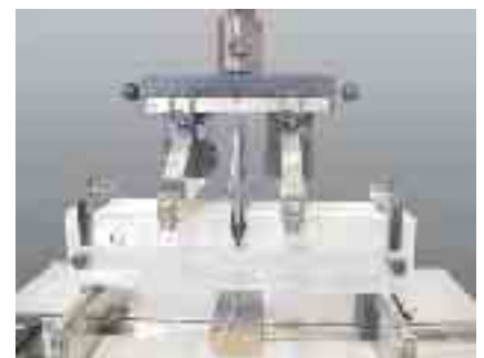
Transducer for measuring the bending deformation
